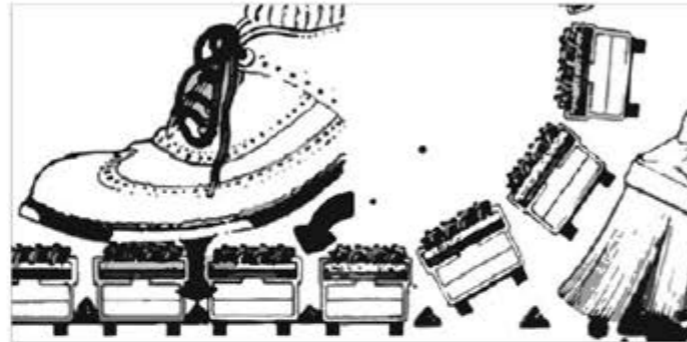
The dirt will fall through the ribs inside the matwell The dirt is kept from sight and gives the entrance a cared-for impression The mat can be rolled up for cleaning
